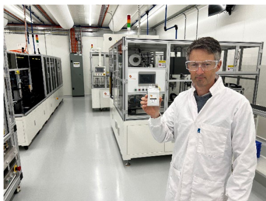
2. Tim Hanley, Li-S Operations Manager holding a 20Ah cell manufactured on the Phase 3 line
